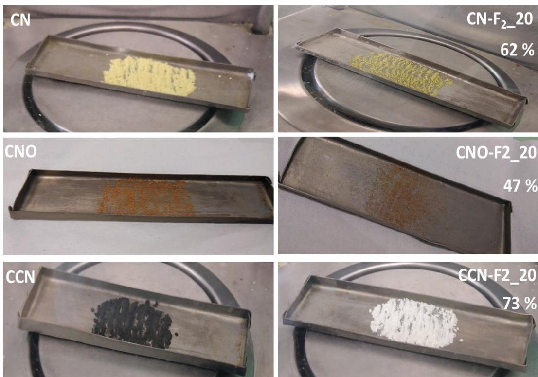
Figure 16. Materials before (left) and after (right) fluorination and their mass gain.
