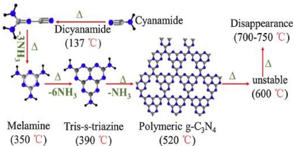
Figure 2. Reaction path of the formation of g- C_3N_4 , starting from cyanamide (reproduced with permission from reference) [51].
